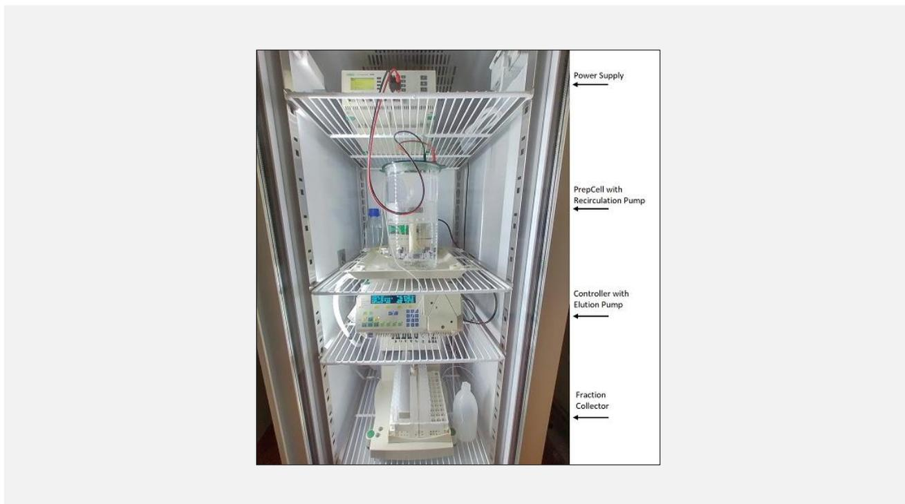
**Figure 1.** The high resolution continuous preparative electrophoresis system consists of a power supply, the preparative electrophoresis cell (PrepCell) with a buffer recirculation pump, a controller with an elution pump, and a fraction collector, all set up in a chromatography refrigerator.
